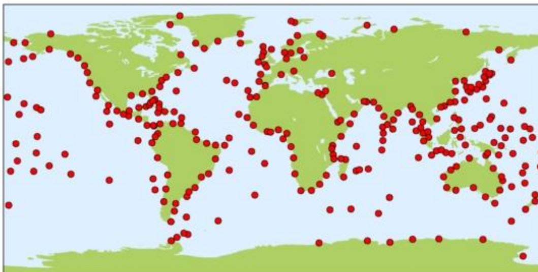
Figure 4.3 GLOSS Core Network of tidal gauges for sea level measurements
