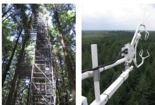
Figure 3.5 Eddy covariance flux tower (courtesy ITC)
